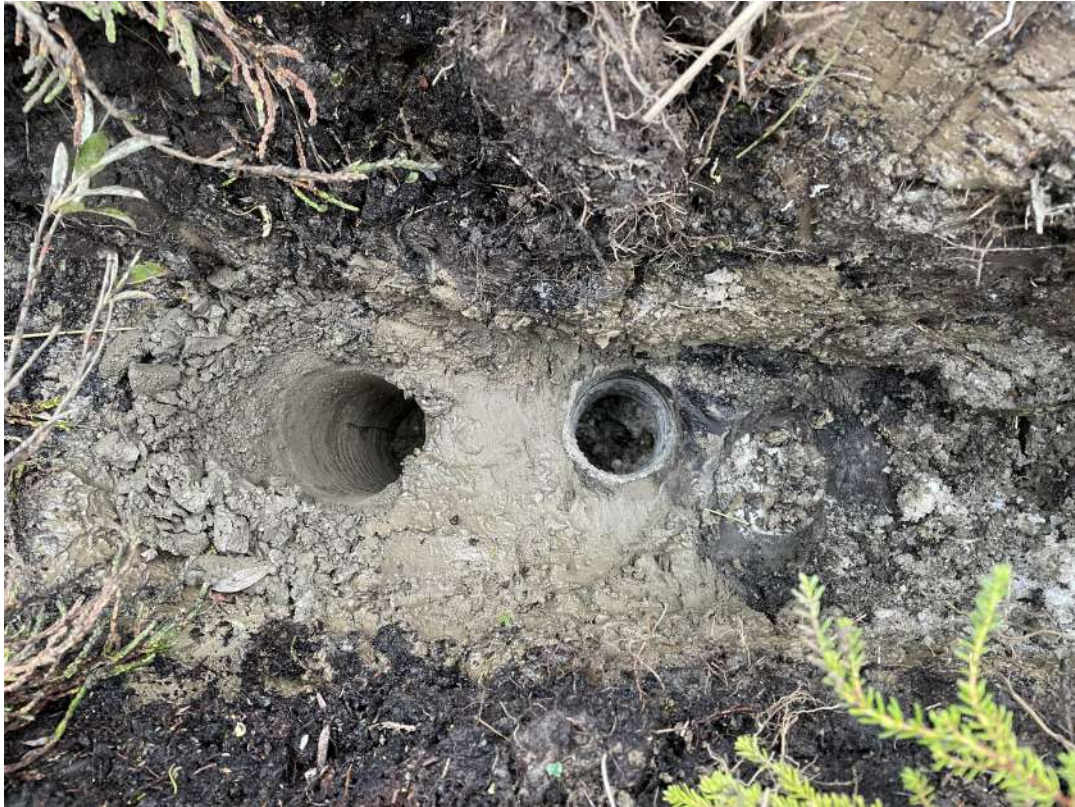
Figure 4.5: Downslope edge of E2. The hole on the right was at the edge of the wedge with the light colour indicating ice along the wall of the drill hole, while the hole on the left did not encounter wedge ice.
